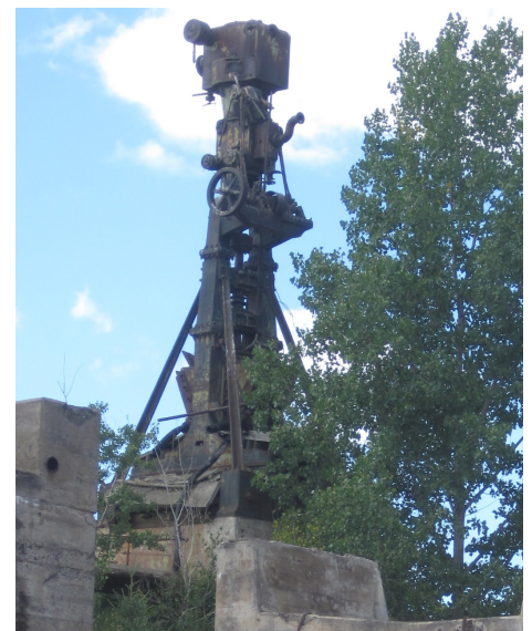
Photograph of last standing steam stamp at the remains of the Ahmeek stamp mill in Tamarack City. (1990).
